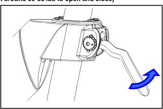
2. Using a 3mm hex wrench, loosen the M6x15 dome screw to free the post handle pin. Loosen the screw about 2-3 full turns, do not remove completely. Push on dome screw to disengage teeth on opposite side.
