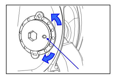
4. Tighten the M6x15 dome screw to secure pin position.
