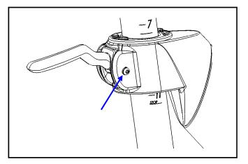
3. Using a 6mm hex wrench, turn the head of the post handle pin. Turn the indicator point on the head of the pin towards the plus sign to add clamp force, or towards the minus sign to remove clamp force. There are each tooth represents a change in clamp force.
