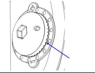
6. Test clamping force by closing handle. The clamp should be set strong enough to hold the user's weight, yet be easy enough for all users to close. Repeat steps 1-6 until desired clamp force is set.
