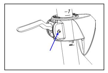
5. Be sure that teeth are fully engages to prevent the post handle pin from losing its position.
